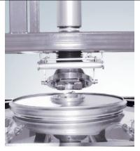
Simple linking of the drive to the stirring unit.
