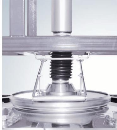
Stirring unit in connected state.
