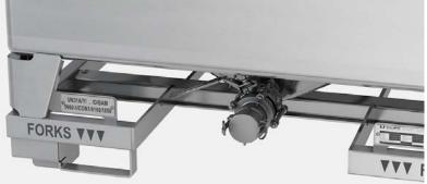
Deep drawn top head and bottom assure high form stability Screw cover with hinge Closing by 6 hammer bolts with wing nuts Robust base frame by additional cross bracings Potential balance between container and support frame by earthing strap.
