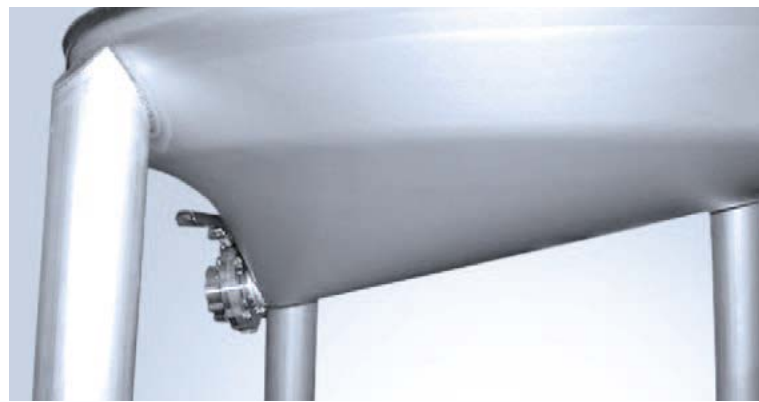
Bottom and outlet recess have been designed in one piece. This avoids the possibility of deposits forming in welded joints.
